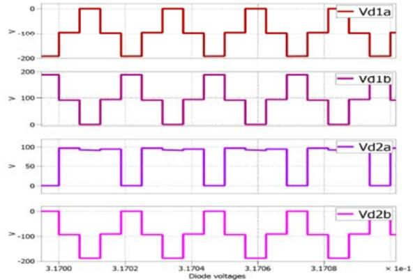
Fig. 7: Simulation result of diode voltage
