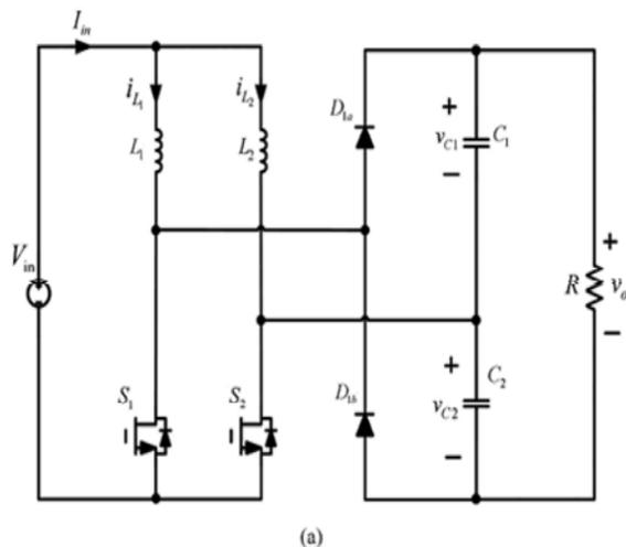
Fig. 2(a): Configuration of two-phase interleaved boost converter
