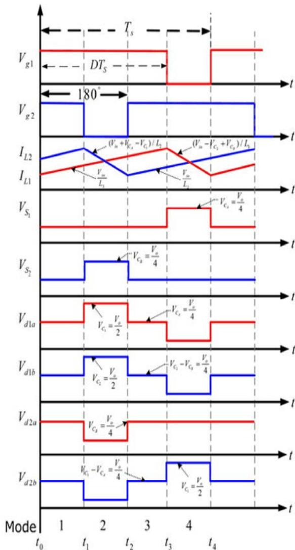
Fig. 3: Operating waveform
