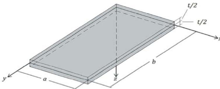
Fig. 1: The coordinate and dimensions of the rectangular plate  $a \times b$  used in the study
