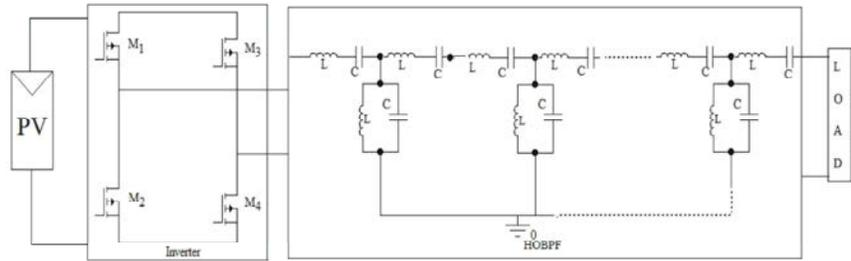
Fig. 5: Applying HOBPF with load.
