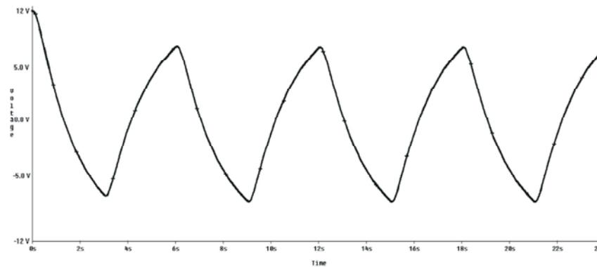
Fig. 9: Output of HOLPF with load.
