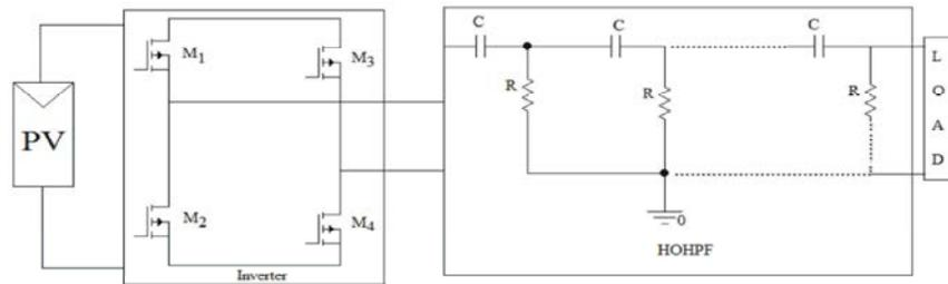
Fig. 4: Applying HOHPF with load.
