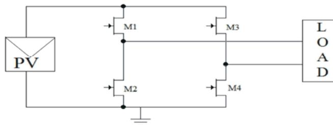
Fig. 2: DC to AC converter with load.
