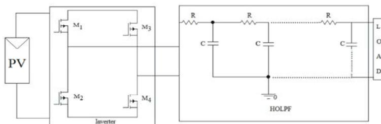
Fig. 3: Applying HOLPF with load.
