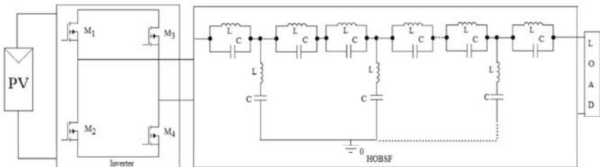
Fig. 6: Applying HOBSF with load.
