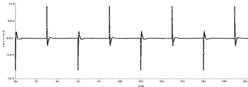
Fig. 10: Output of HOHPF without load.
