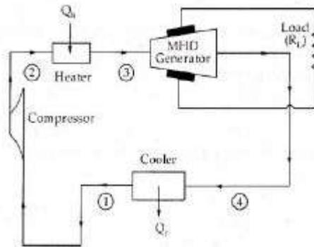
Fig. 6: Power cycle for MHD generator
