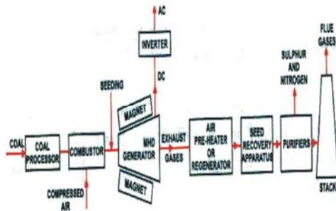
Fig. 7: An open cycle Coal fired MHD system
