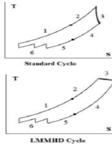
Fig. 12: Comparison of Standard Brayton cycle with with MHD Brayton cycle
