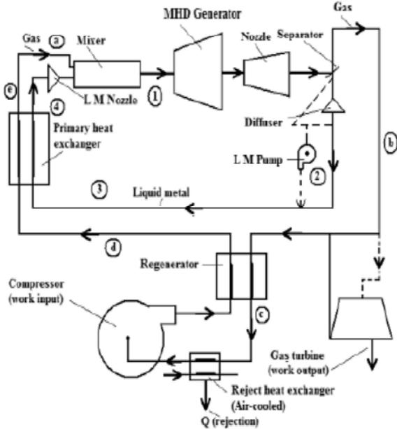
Fig. 11: Schematic two-phase cycle LMMHDEC system
