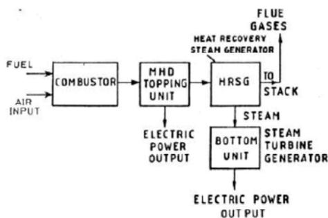
Fig. 9: A coal fired, MHD topping unit with steam turbine bottom unit.
