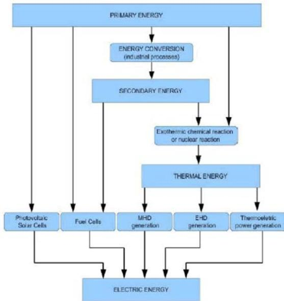
Fig. 1: Direct energy conversion stages [1].
