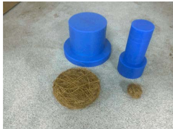
Fig. 2: Plastic moulds and date palm fiber samples
