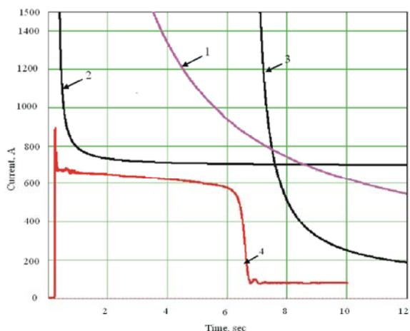
Fig. 2: Comparison of suggested current-time curve with existing protection
