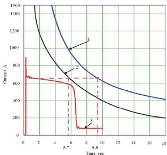
Fig. 1: Starting and protection performance of high-voltage electric motor air turbocharger: 1 – current characteristic; 2 – offered feature 3 – starting characteristic
