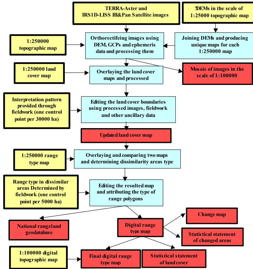
Fig. 1: Processes flowchart of the project. Yellow, blue and red boxes are Inputs, Processes and Outputs respectively
