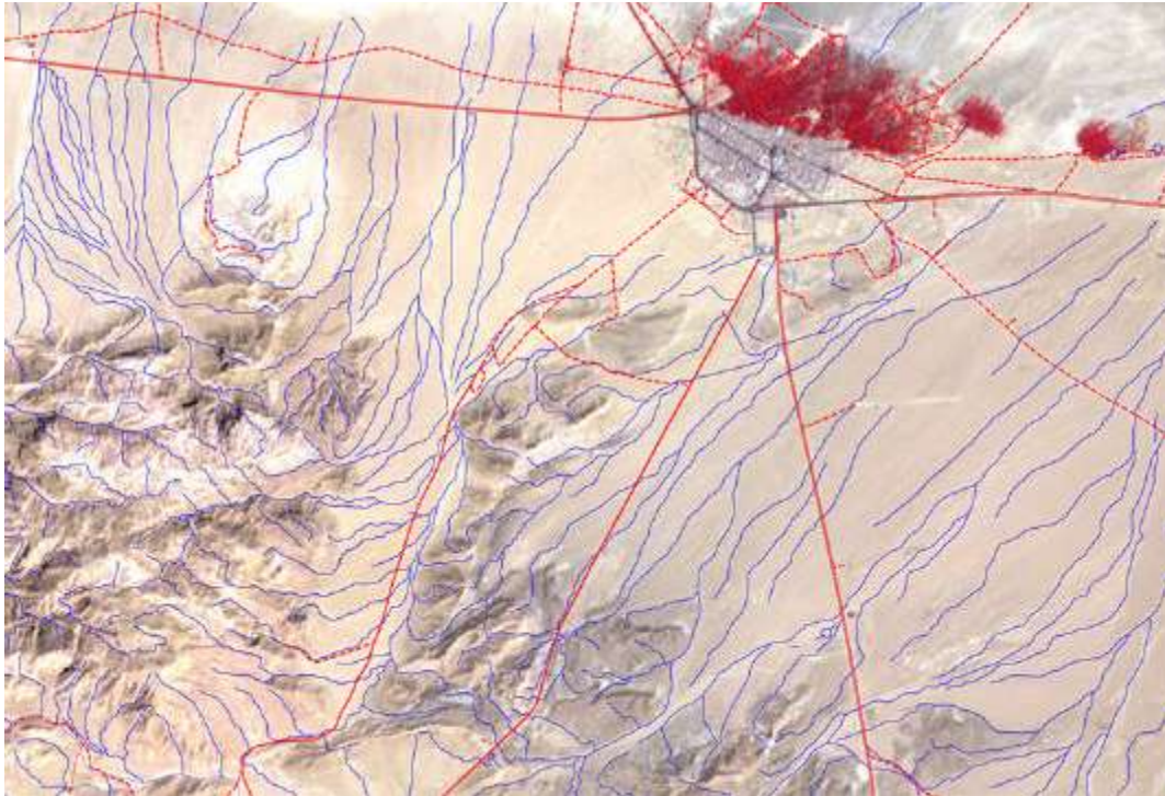
Fig. 4: High precision of orthorectified image, in compare with roads and rivers
