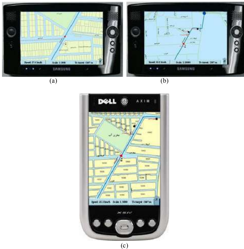
Fig. 2: Generated maps using context-aware car navigation system; a) speed < 20 km/h and screen size=7 inches, b) speed > 50km/h and screen size= 7 inches, c) speed < 50km/h and screen size= 3.7 inches
