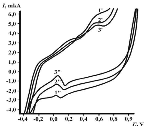
Fig. 1: Cyclic voltammetric curves for GE-Au<sub>nano</sub>: 1', 1''- 0.1 M NaOH background solution; 2', 2''- presence of  $2 \cdot 10^{-12}$  M cysteine; 3', 3'' - presence of  $4 \cdot 10^{-12}$  M cysteine.
