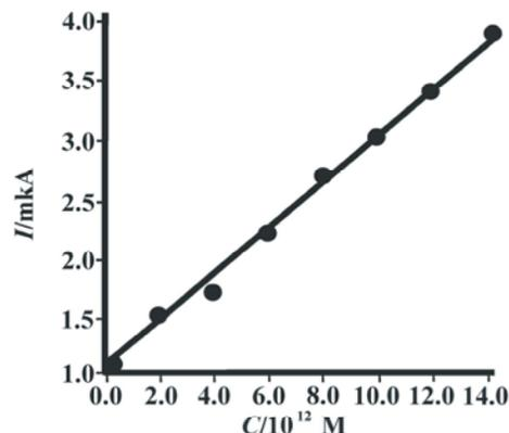
Fig. 2: Dependence of the maximum oxidation current on cysteine concentration on the GE-Au-nano in 0.1 M NaOH solution.
