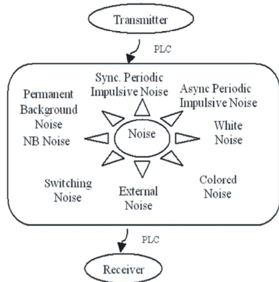
Fig. 2: Expected Noise in the transmission for SG
