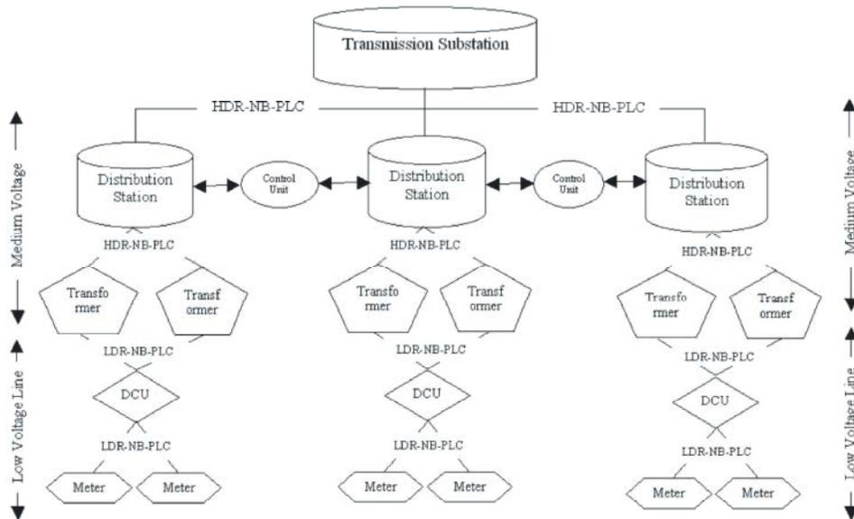
Fig. 1: Proposed PLC Network Topology
