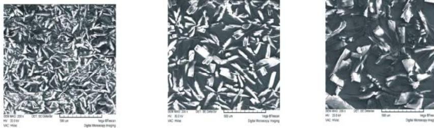
a) Sand blasting phosphating (S-Ph)    b) Grinding phosphating (G-Ph)    c) Shot blasting phosphating (Sh-Ph)
