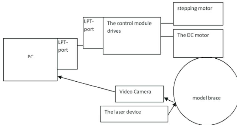
Fig. 3: The scheme of connecting devices to a personal computer
