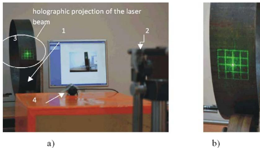
Fig. 2: Stand assembly (a) and view the projected figure (b) on the surface of the shroud model
