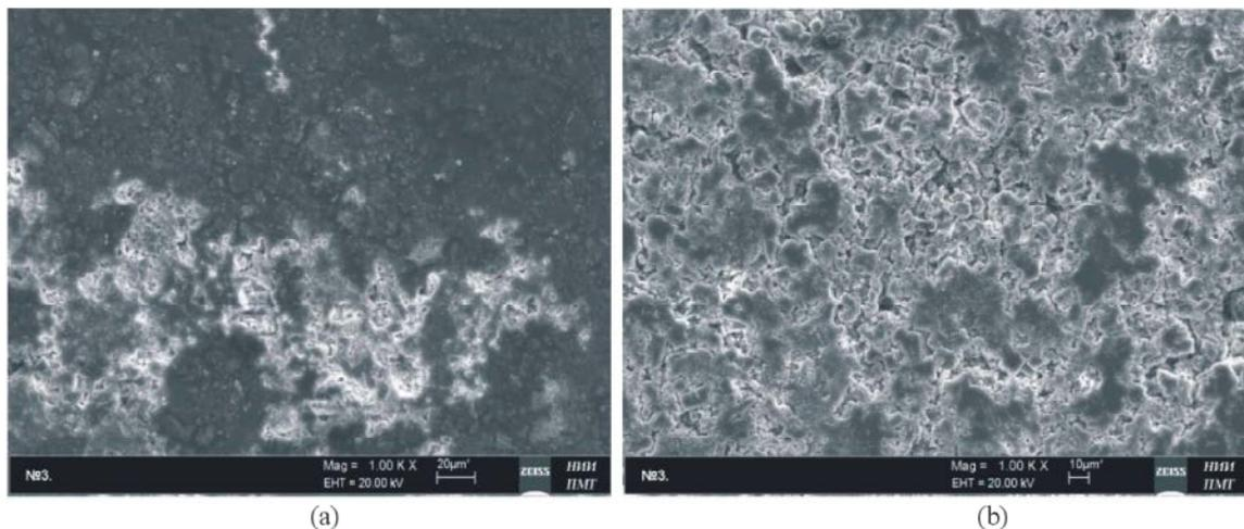
Fig. 6: The SEM-image of the surface morphology of composite with 70 mas. % of modified  $[\alpha]\text{-Al}_2\text{O}_3$  a) untreated and b) treated with oxygen plasma flow
