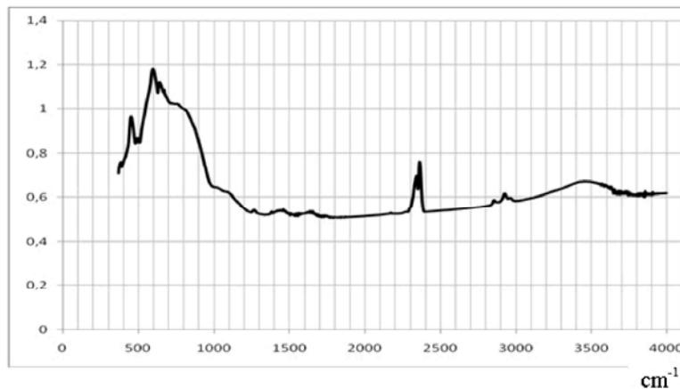
Fig. 2: FT-IR spectrum of the synthesized modified [alpha]-Al<sub>2</sub>O<sub>3</sub>
