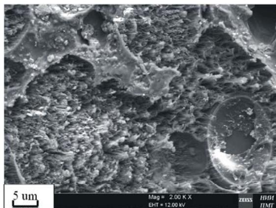
Fig. 4: SEM-image of the surface morphology of polystyrene, treated with oxygen plasma beam
