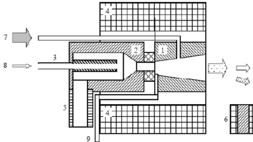
Fig. 1: Scheme of magnetoplasmadynamic accelerator: 1-anode; 2-ferromagnetic intermediate electrode; 3-hollow hot cathode; 4-solenoid; 5-additional vacuum pumping duct; 6-deflection electromagnet; 7-plasma-supporting gas pipe; 8-inert gas pipe; 9-feed route of protective gas H<sub>2</sub>
