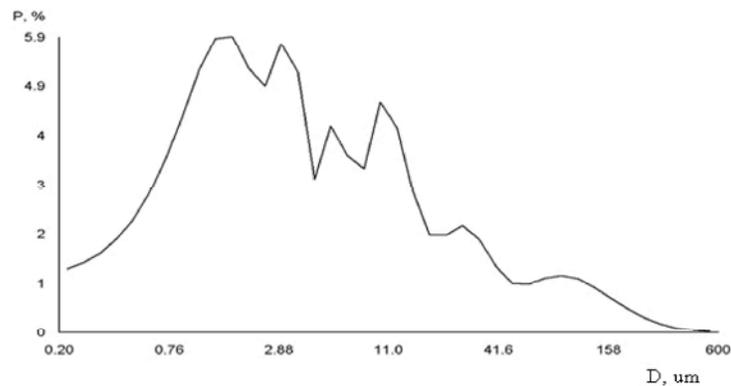
Fig. 3: Granulometric composition of the synthesized modified [alpha]-Al<sub>2</sub>O<sub>3</sub>
