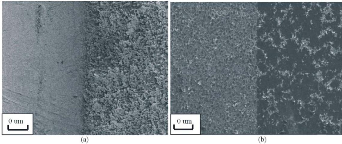
Fig. 5: The image of the border between the untreated area and area treated with oxygen plasma flow: a-pure polystyrene sample; b-polystyrene composite with 70 mas. % of modified  $[\alpha]\text{-Al}_2\text{O}_3$ .
