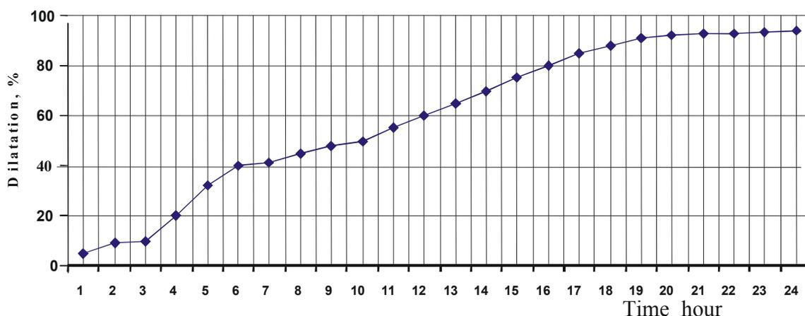
Fig. 4: Volume of the expanding deformation composition
