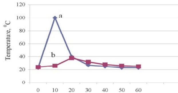
Fig. 2: Hydration activity dolomitic lime obtained by calcining at 900° C: no additive (a); with the addition of Na<sub>2</sub>CO<sub>3</sub> (b)
