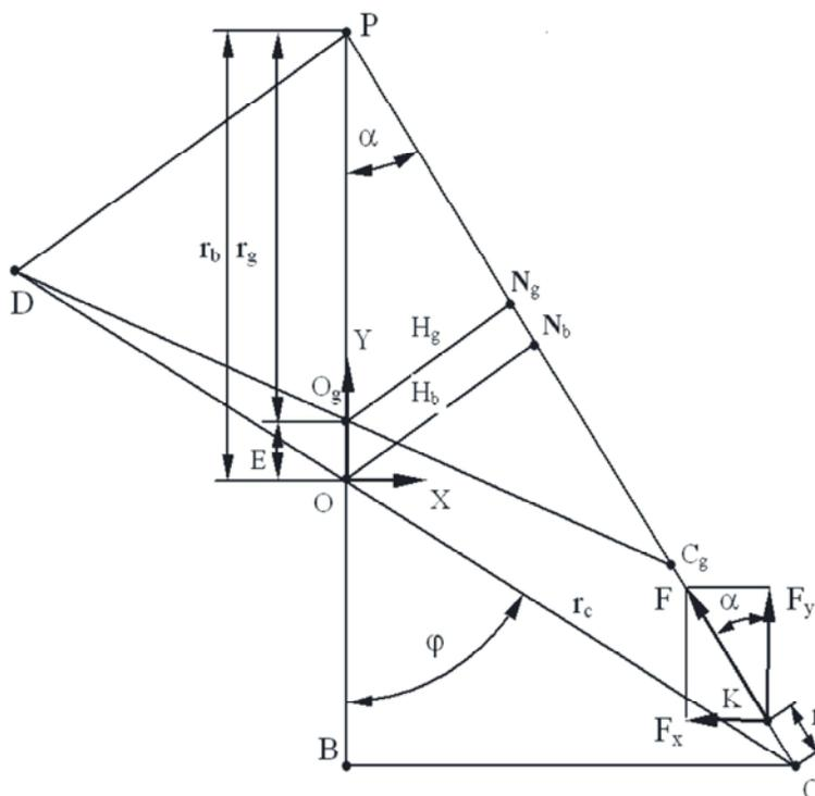
Fig. 2: Bobillier construction and force in the ring gear pin engagement with the satellite tooth:
