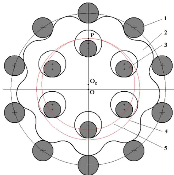
Fig. 1: Gear-pin cycloid reducer:
