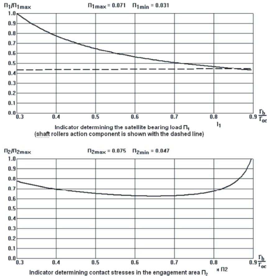
Fig. 3. Dependency of  $\Pi_1$  и  $\Pi_2$  indicators on the  $\frac{r_b}{r_{oc}}$  ratio
