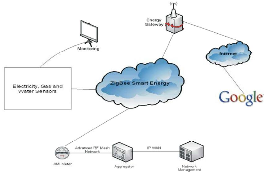
Fig. 4: Data Communication of AMI using ZigBee
