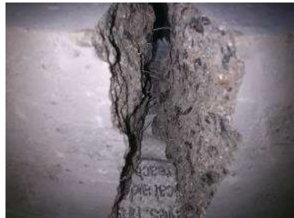
Fig. 13: Effective fibre bridging – pullout resistance
