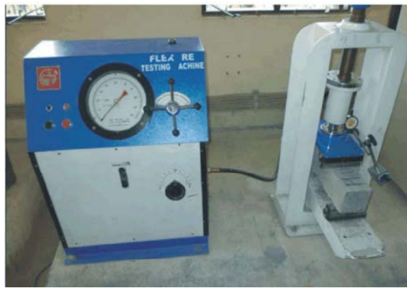
Fig. 4: Test setup for flexural testing machine
