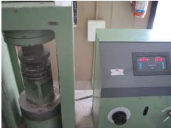
Fig. 3: Test setup for compressive testing machine
