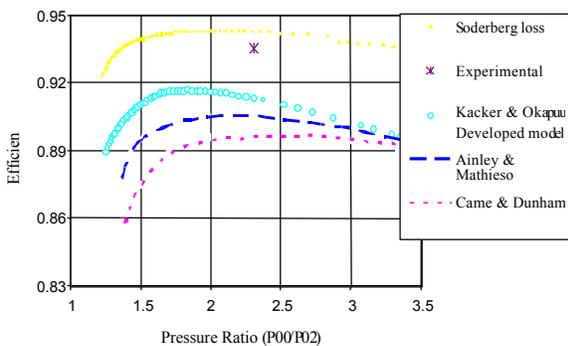
Fig. 8: Comparison between predicted efficiencies and experimental data at 5041 rpm
