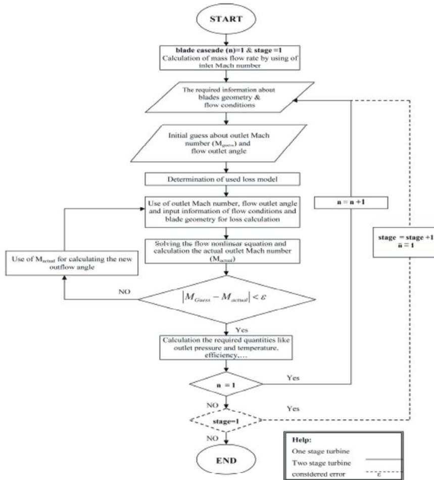
Fig. 1. Suggested algorithm for turbine 1D modeling
