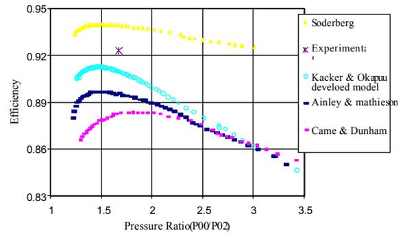
Fig. 9: Comparison between predicted efficiencies and experimental data at 4030 rpm
