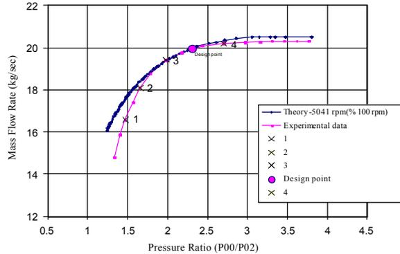
Fig. 5: Mass flow v s. Pressure ratio at design speed by using of Kacker and Okapuu's developed model
