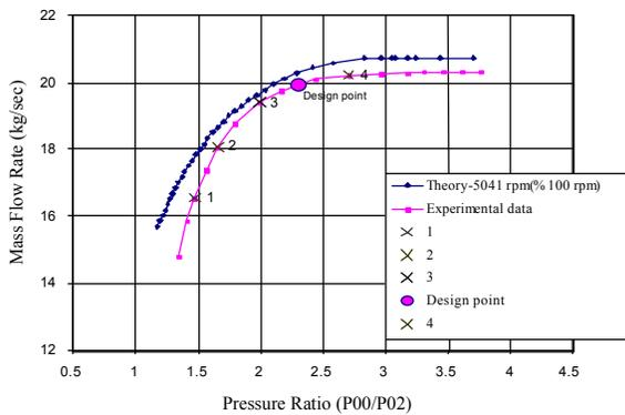
Fig. 2: Mass flow vs. Pressure ratio at design speed by using of soderberg's model
