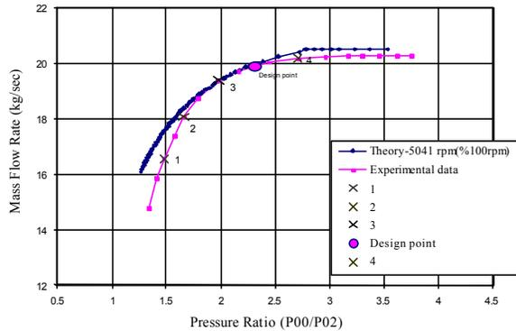
Fig. 3: Mass flow vs. Pressure ratio at design speed by using of Ainley & Mathieson's model
