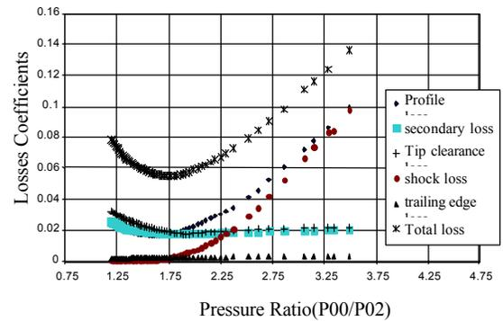
Fig. 10: Loss coefficients vs. Pressure ratio
