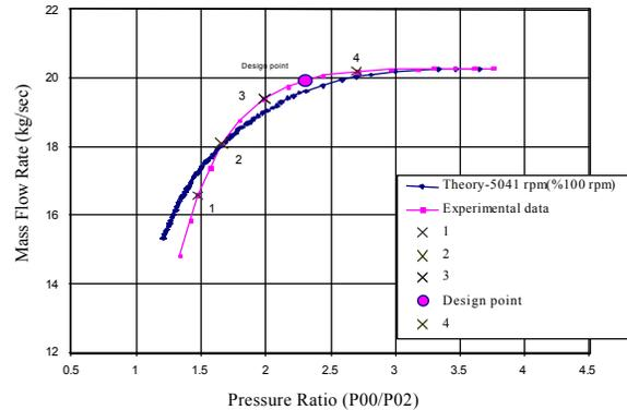
Fig. 4: Mass flow vs Pressure ratio at design speed by using of Came & Dunham's model
