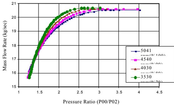
Fig. 6: Mass flow vs. Pressure ratio at different rpm
