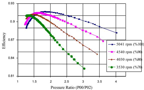
Fig. 7: Turbine efficiency vs. Pressure ratio at different rpm
