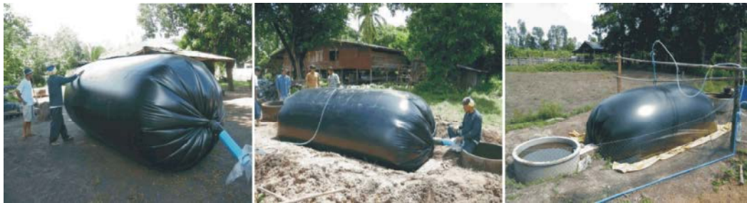
Fig. 2: Balloon biogas technology from PVC plastic
