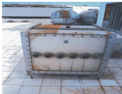
Fig. 11: Test-rig (A) after a period of operation with buckling, as well as cracks
