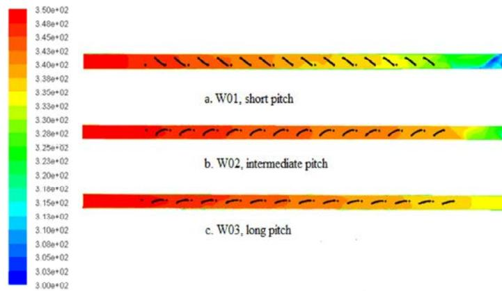
Fig. 7: Water temperature inside tube for three different type of coils
