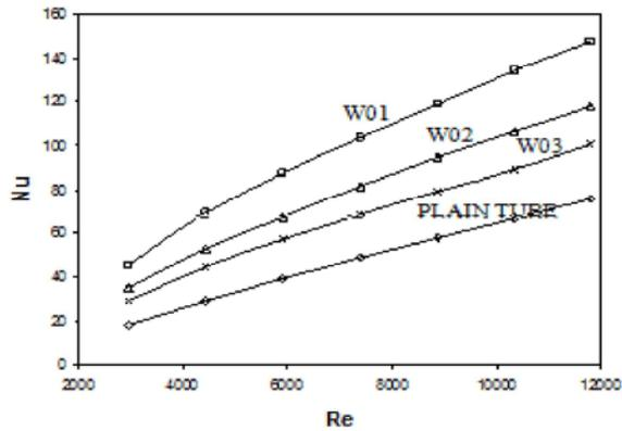
Fig. 3: Nusselt number versus Reynolds number in different cases of tubes with wire coils tube wire less
