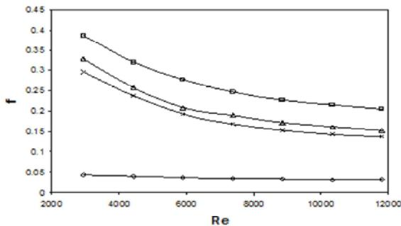
Fig. 4: Friction coefficient versus Reynolds number in different cases of tubes with wire coils tube wire less
