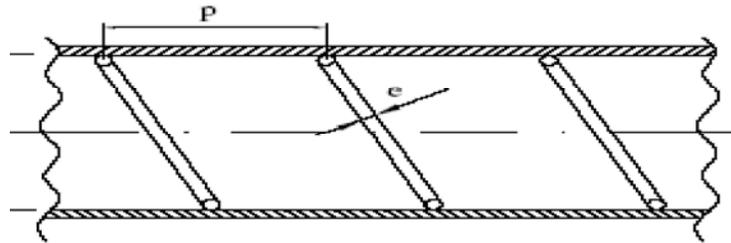
Fig. 1: View of the tubes and wire coils inserts and their dimensions
