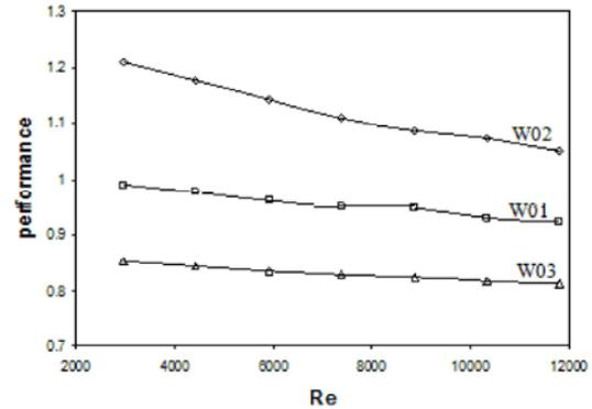
Fig. 5: Performance coefficient versus Reynolds number in different cases of tubes with wire coils tube wire less
