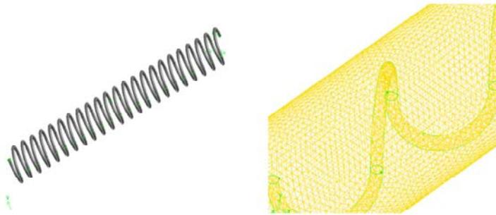
Fig. 6: A view of coil inserts and its mesh
