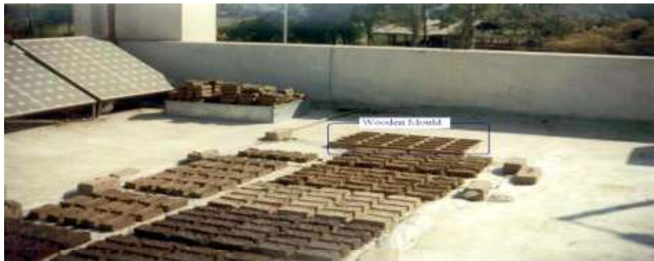
Fig. 9: Moulding (Wooden Mould outlined ) and drying of briquettes
