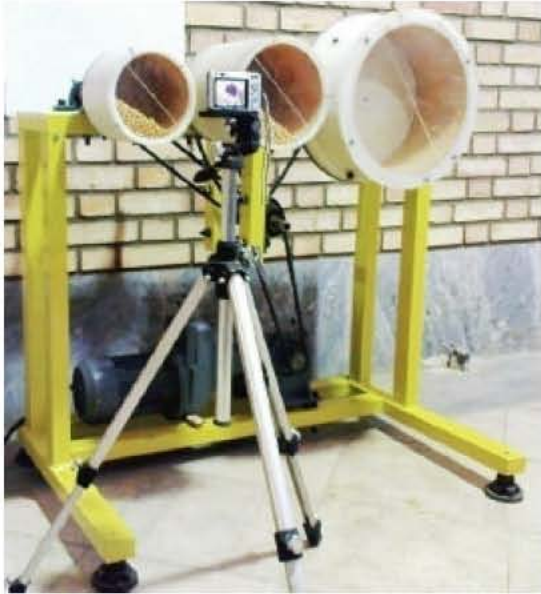
Fig. 3: Apparatus for measuring the angles of repose
