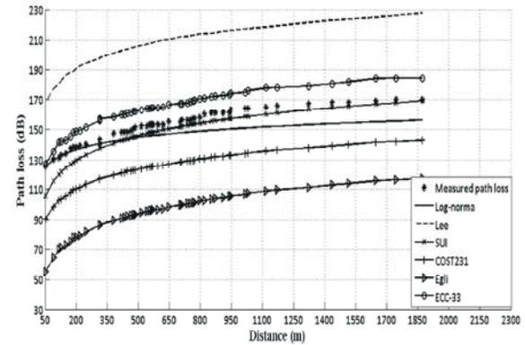
Fig. 4: Comparison between measured path loss and that predicted by using empirical models for T4
