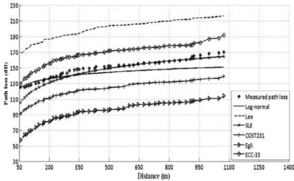
Fig. 1: Comparison between measured path loss and that predicted by using empirical models for T1
