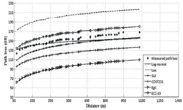
Fig. 3: Comparison between measured path loss and that predicted by using empirical models for T3
