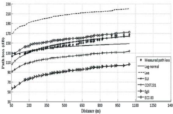
Fig. 2: Comparison between measured path loss and that predicted by using empirical models for T2
