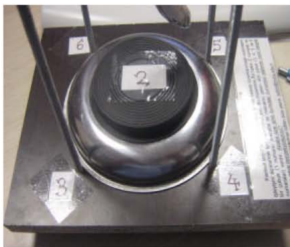
Photograph 2: The pendulum mechanism which consist of one of them big (number 2) and one of them tied up to a rope (number 1) magnet and four steel bar (number 3,4,5 and 6) that is used for explaining the chaos theory.
