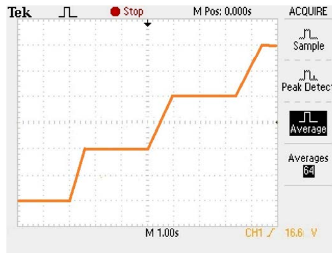
Fig. 7: (a) Experimental setup for ANFIS based rotor position controller, (b) Ramp rotor position response of BLDC motor, (c) Step rotor position response of BLDC motor
