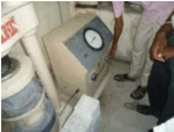
Fig. 2: Compressive Strength Test Setup
