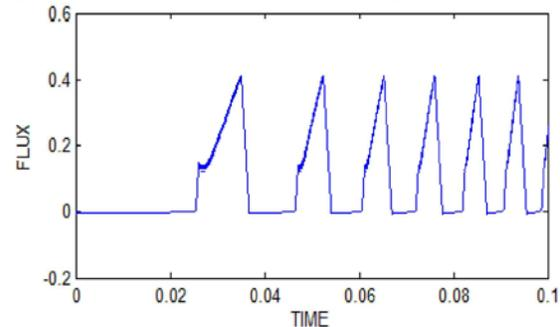
Fig. 7.3: Motor Flux linkage waveforms of open loop control
