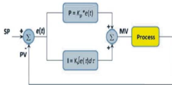
Fig. 5.1: Basic block of a PI controller
