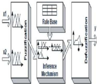
Fig. 6.1: Block diagram of SRM speed control
