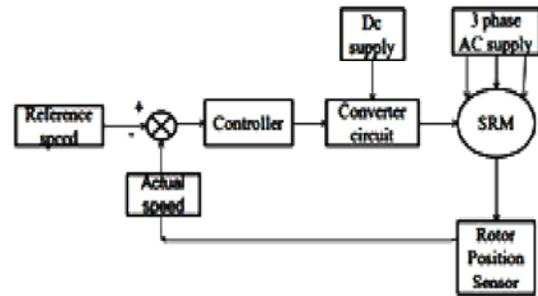
Fig. 4.1: Block diagram of SRM speed control.
