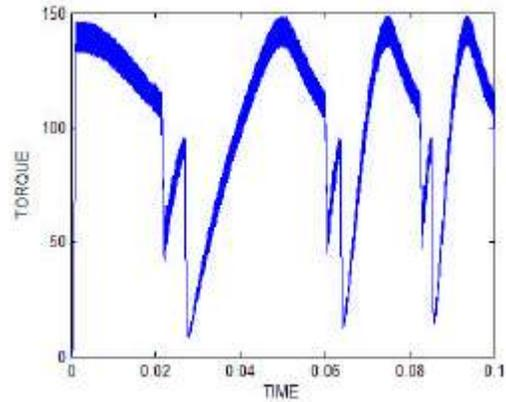
Fig. 7.8: Motor Torque waveforms of closed loop control using PI controller
