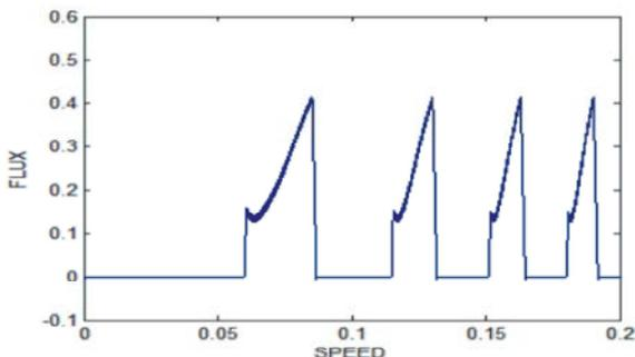
Motor Flux Linkage Waveforms of Closed Loop Control Using PI Controller:
