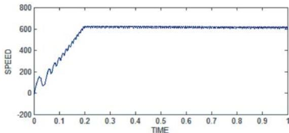
Fig. 7.7: Motor Speed waveforms of Closed loop control using PI controller
