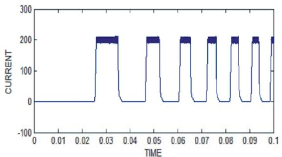
Fig. 7.4: Motor current waveforms of open loop control
