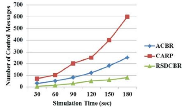
Fig. 4: Routing Overhead with respect to Simulation time
