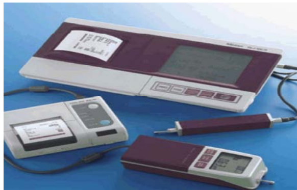
Fig. 4: Surface roughness measuring instrument (SJ 201)
