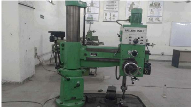
Fig. 1: Drilling Setup (BVR 3)
