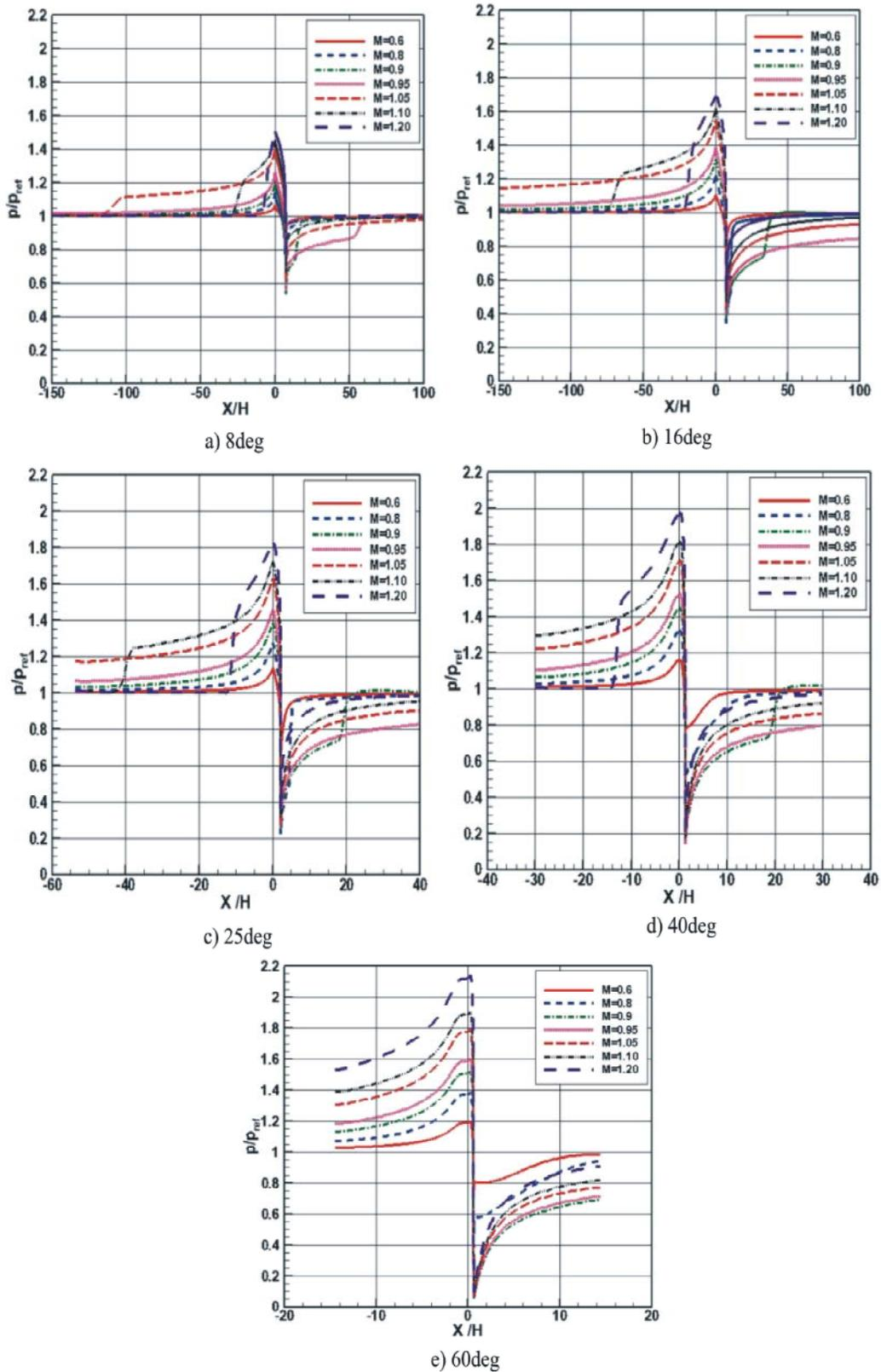
Fig. 4.2: Pressure Distributions over Various Compression Corner at Transonic Mach number
