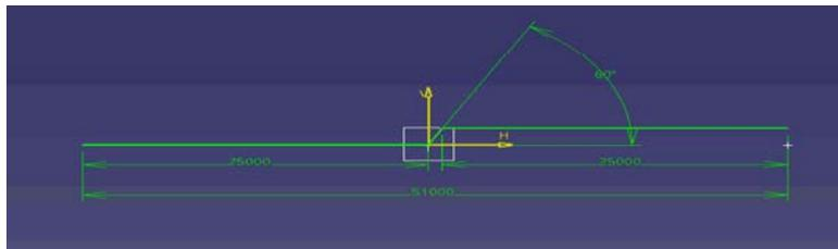
Fig. 2.1: Ramp angle of 60deg
