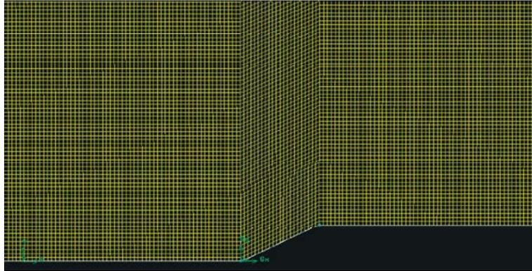
Fig. 3.1: Meshed View of Compression Ramp
