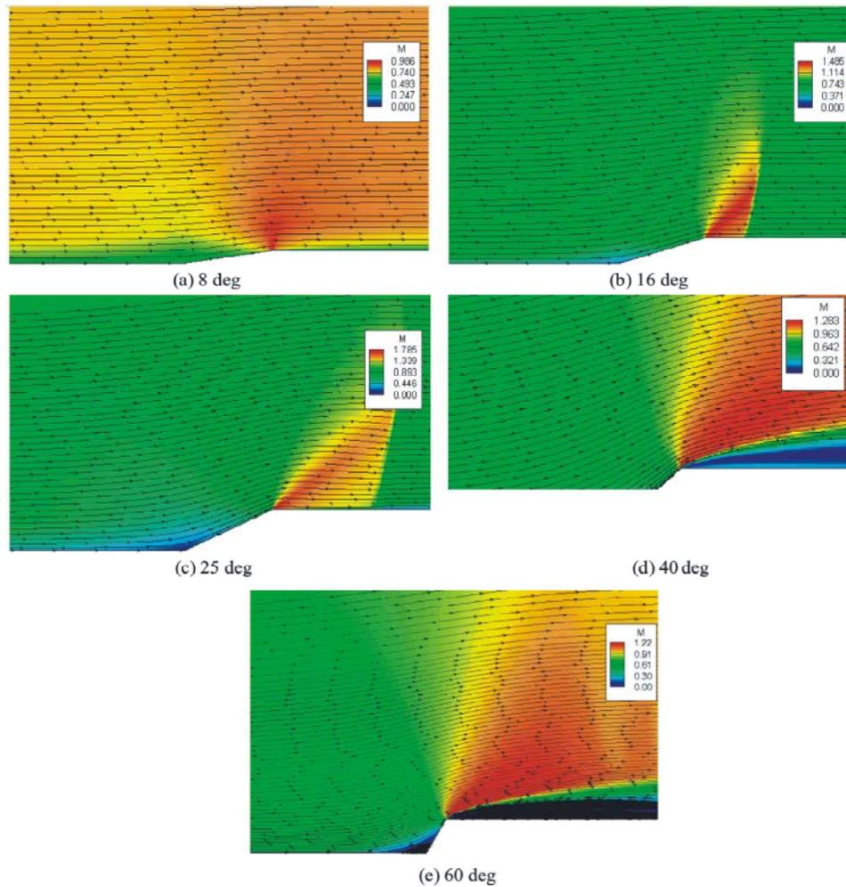
Fig. 4.3: Mach Palette with Streamlines for Various Compression Corner Angles at M=0.8
