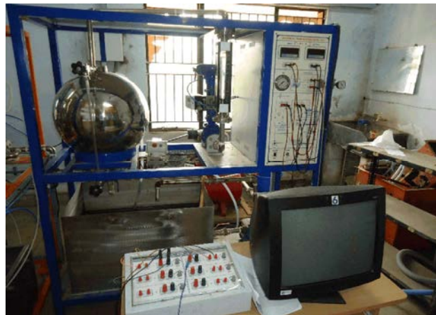
Fig. 3: Real Time Laboratory setup for Spherical Tank Process
