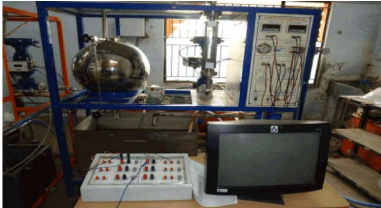
Fig. 2: Experimental set up for a spherical tank
