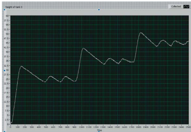
Fig. 11: Response of Closed Loop controlled by PID controller
