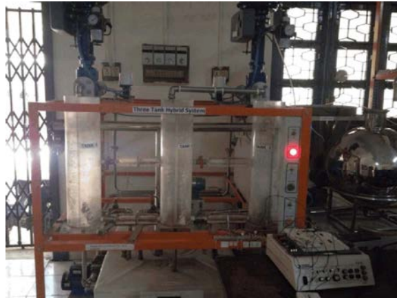
Fig. 1: Laboratory setup of the three tank interacting system
