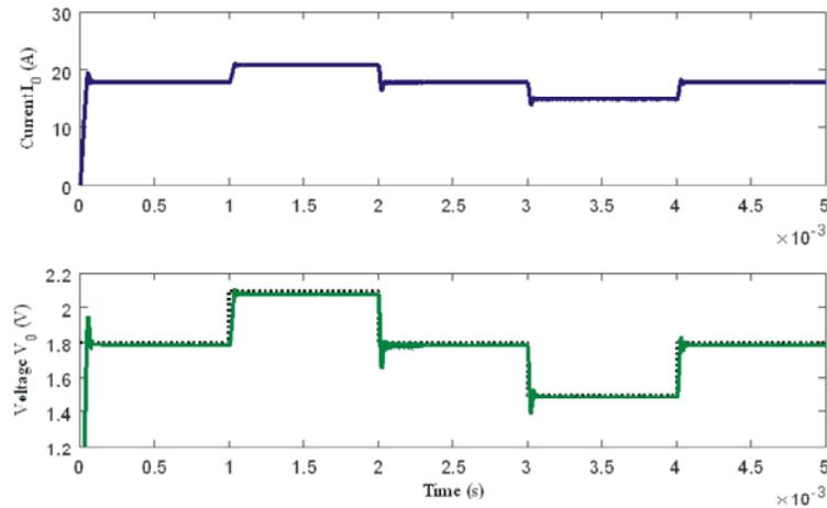
Fig. 9: Simulated output voltage with line disturbances (1.8V-2.1V-1.8V) under nominal load 100 Ω
