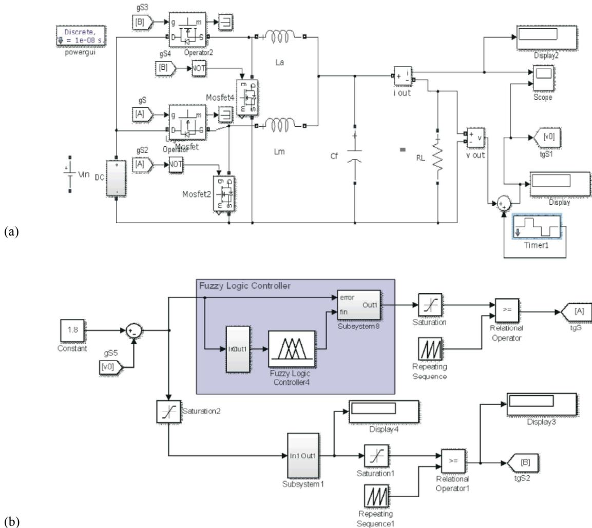
Fig. 7: (a) Overall Simulink of FRDB converter using fuzzy logic control (b) Fuzzy logic controller duty control
