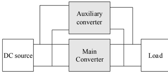
Fig. 1: Structure of fast response double buck converter
