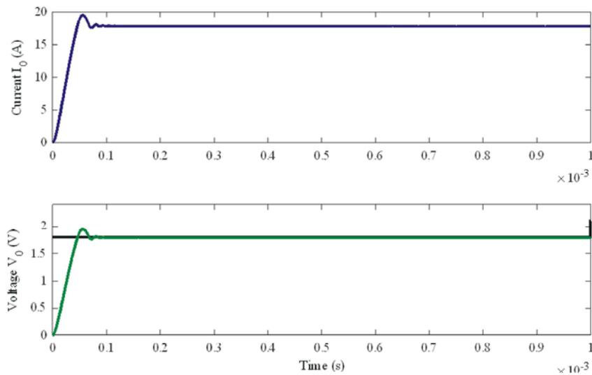
Fig. 8: Simulated start-up of the output voltage and current with set point 1.8V and nominal load  $100\Omega$
