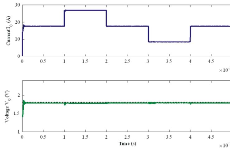
Fig. 10: Simulated output voltage with load disturbances (18A -28A -18A)
