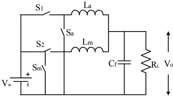
Fig. 2: Circuit diagram of fast response double buck converter
