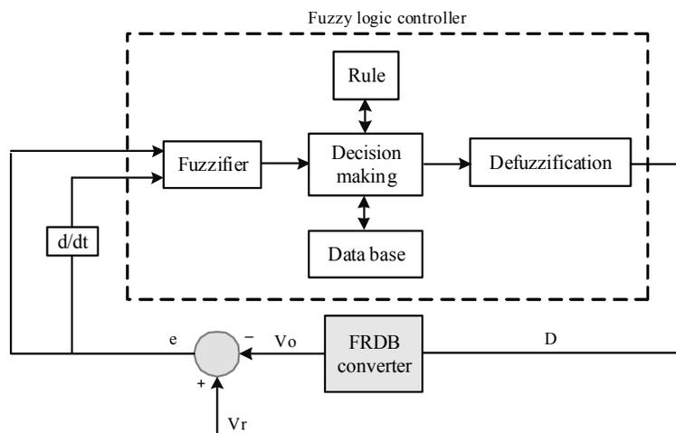
Fig. 3: Block diagram of fuzzy logic controller
