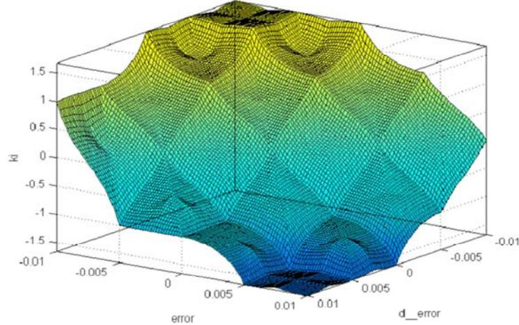
Fig. 5: Fuzzy Integral gain response over error and change in error
