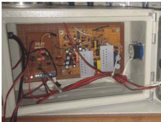
Fig. 4: Circuit Box of the Digital Absolang
