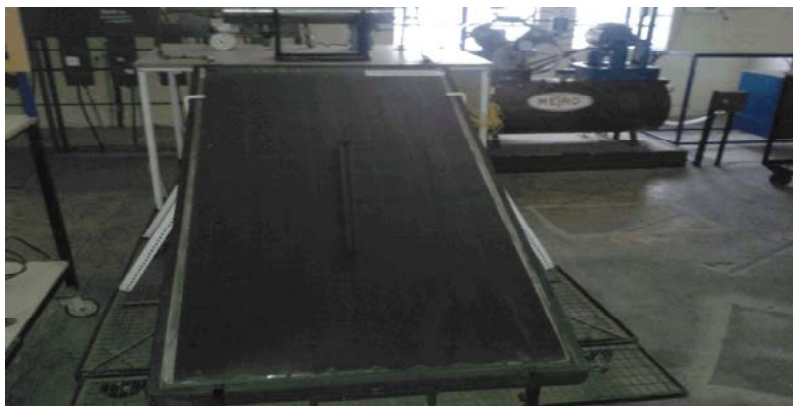
Fig 1: Experimental setup of solar flat-plate collector
