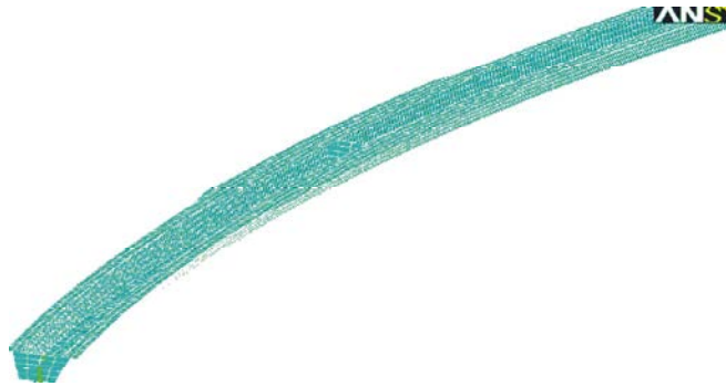
Fig. 14: 3D-FEM for three spans horizontally curved continuous box girder with horizontal XD type truss.
