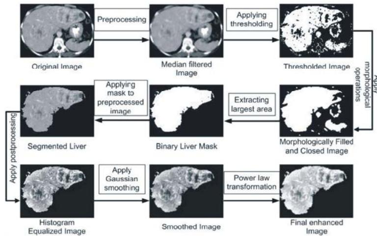
Fig. 1: Flow diagram of Computerized System for Liver CT Segmentation and Enhancement
