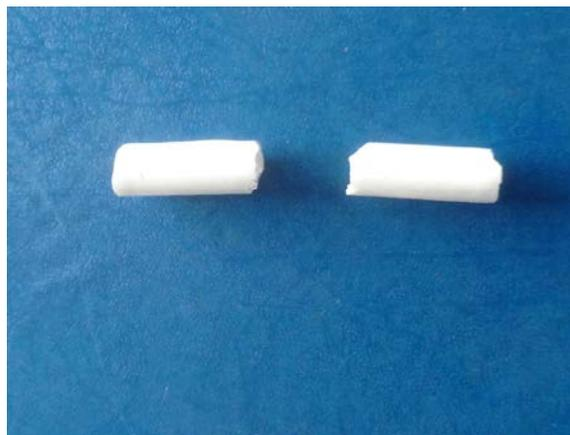
Fig. 1:  $\text{TiO}_2$  powder on glass tubes catalysts.
