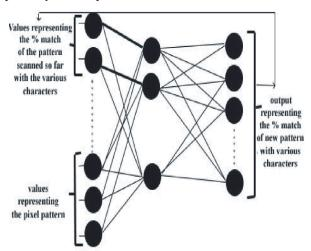
The Custom-Made Neural Network Architecture: The proposed idea for recognizing the handwritten document demand a network where in the state transition during the analysis of each column of pixels could be represented. So we propose a new architecture of neural network that would suit this need. The network that we propose would accept inputs in each layer. The network would have more hidden layers than the maximum number of pixels forming the width of the characters [9].
