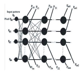
But these hidden layers do not behave exactly as hidden layers in the fact that they take inputs too. The output of each layer would depend on the input it receives from the previous layer as well as the input representing the pixel pattern.
