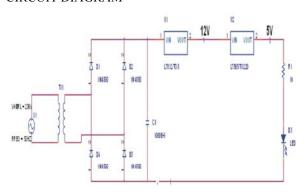
obtained from the output pin of 7805 is fed as the supply to the micro controller. From the same output pin of the 7805, a LED is connected in series with the resistor to indicate that the power is ON.
