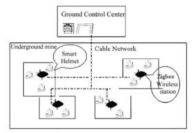
Fig. 1: Structure of the system
