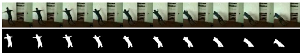
Fig. 3: Images from top left to the right show 89 to 99 frames of a sample video sequence from the fall of an individual and in the bottom column, the images produced after using Gaussian mixture model and thresholding has been presented in binary format.
