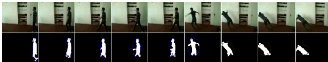
Fig. 5: Images from top left to the right, 40, 45, 53, 61, 66, 89, 95, 97 and 99 frame and in bottom columns from left to the right, the change of oval based on variation in one's posture has been depicted and C_{motion} has crossed the defined threshold in frame 95.
