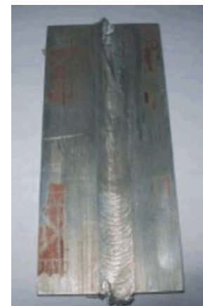
Fig. 8: Friction stir welded aluminum alloy H20 down without preheating and up with 250 C preheating.
