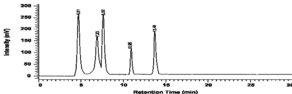
Fig. 3: HPLC Chromatogram of Honey sample: 10.96 Gentamycin Residue, other peaks at 4.61, 7.23, 8.02, 13.49 not identified.
