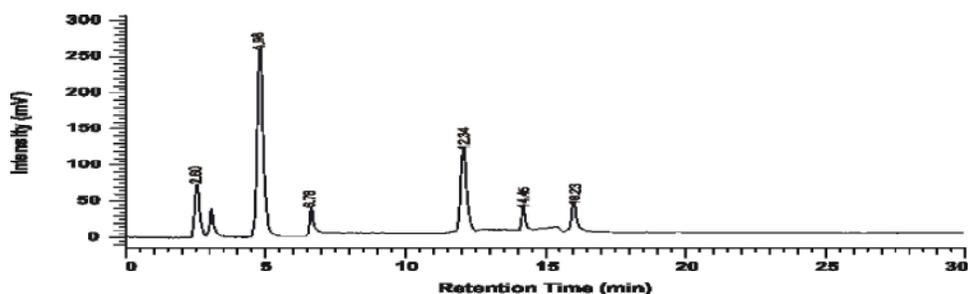
Fig. 2: HPLC Chromatogram of Honey sample: 2.60 Streptomycin Residue, other peaks at 4.98, 6.78, 12.34, 14.45 and 16.23 not identified.
