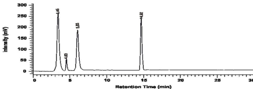
Fig. 1: HPLC Chromatogram of Honey sample: 5.63 Tetracycline Residue, other peaks at 3.45, 4.63, 14.92 not identified
