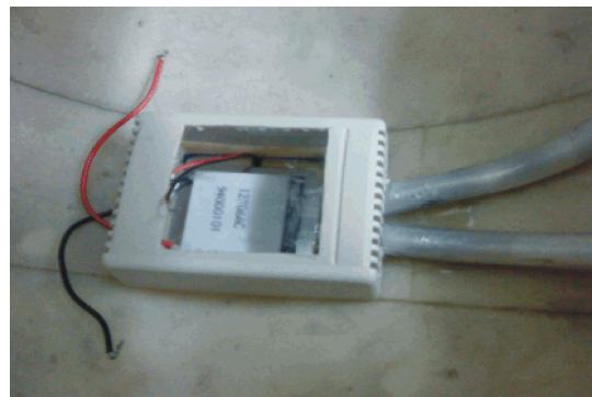
Fig. 2: Aluminum pipe and cooling chamber
