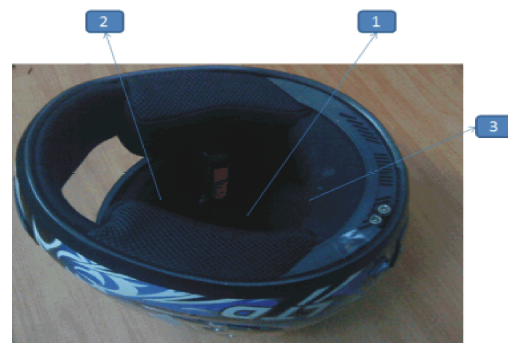
Fig. 12: Thermocouple placement point
