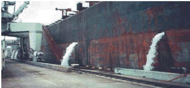
Fig. 2: A photograph shows the discharge of ballast water from a container ship [10]
