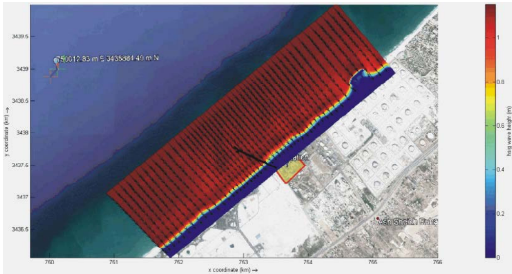
Fig. 12: Wave distribution according to wave height 1.15m & Time period 6sec & Northern west direction
