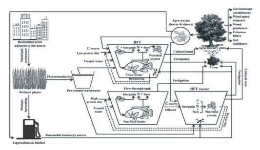
Fig. 1: A large scale application design proposed for wastewater-aquaculture-agriculture integration in arid and semi-arid regions.
