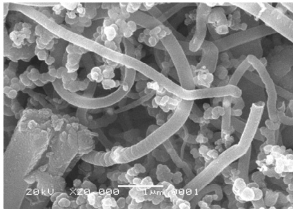
Fig. 2: Cross-sectional FESEM images of modified multi walled carbon nanotubes (MWNTs)
